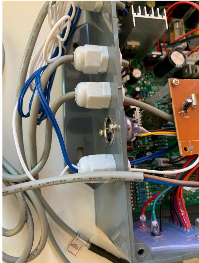
Now Locate the 4 wired plug on the PCB (you can trace these 4 wires from the round DIN type plug)...
